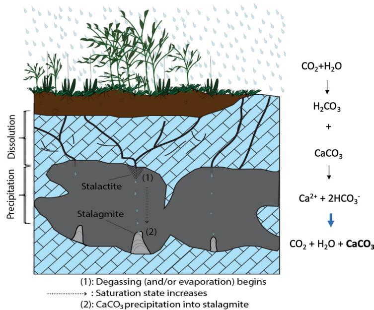
**Figure 7.** Generalized sketch showing the processes of stalagmite formation (from dissolution, degassing and/or evaporation of the drip water, to CaCO<sub>3</sub> precipitation to stalagmite), and the linkage between the cave system and the landscape above it. Stalactite and stalagmite are examples of cave deposits. (Source: Voarintsoa, 2017).
